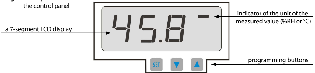
Fig. 8. Description of the control panel
