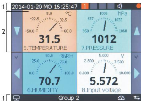
Fig. 11.4. Appearance of a measurement group screen in the ANALOG INDICATOR (counter) mode (presentation max. 6 chan.)
